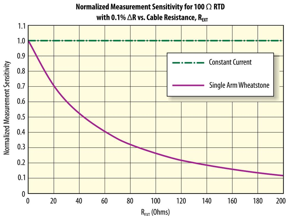
**Figure 2:** Normalized Measurement Sensitivity vs.  $R_{EXT}$
