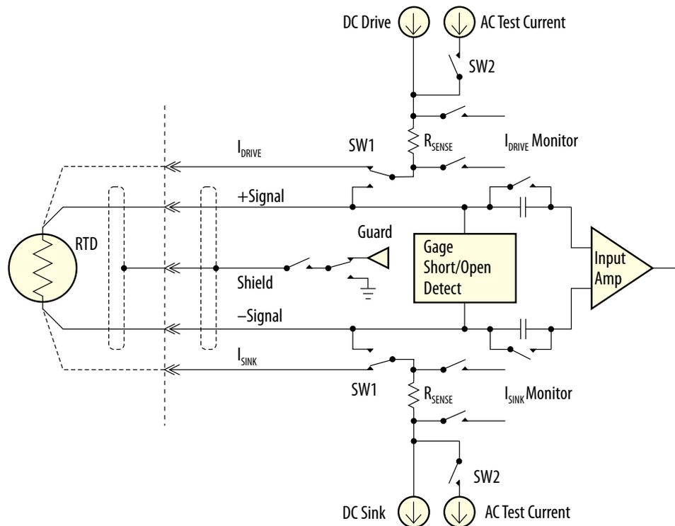
**Figure 5:** Balanced Constant Current Excitation Circuit Diagram
