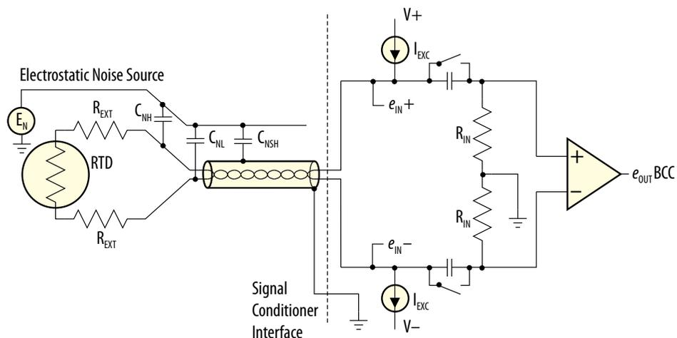
**Figure 4:** Balanced Constant Current Excitation Circuit
