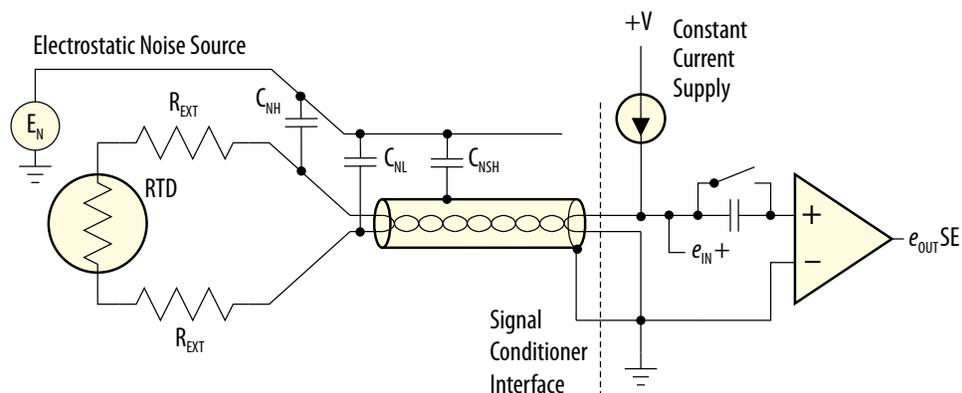
**Figure 3:** Single-Ended Constant Current Excitation Circuit
