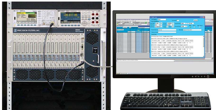
Typical installation with 28016 chassis with 28000-BIF1-FT controller installed, controlled by the 28000 GUI, rack mounted with Keysight Signal Generator and DVM.
