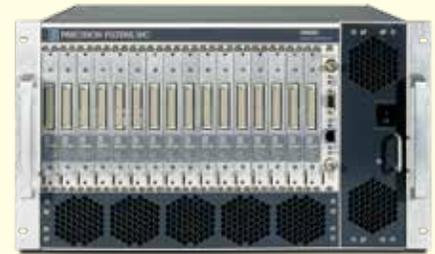
**Qty. 8 28016 Mainframes with Power Supplies and 28000F-BIF1-FT Control Cards with Built-In Test Support**
