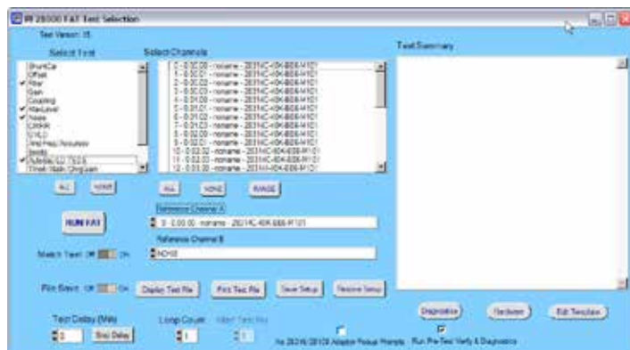
The FAT test selection panel allows the user to select any tests to run on any set of channels. Test results can be saved to a file for later retrieval. A test summary is listed for quick diagnosis.
