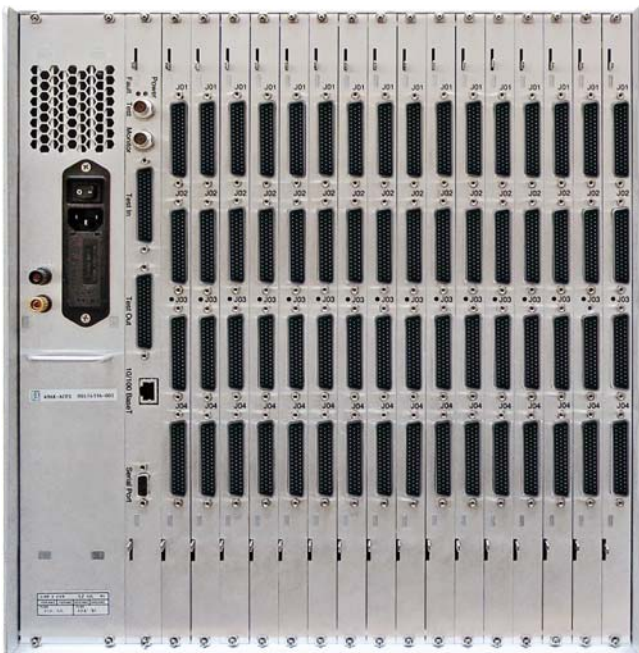
Figure 8 464kB-R1 w/Input Cards and Output Cards Installed
