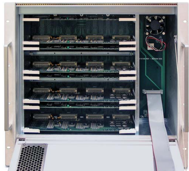
Figure 10 464kB Interstage Cards Installed
