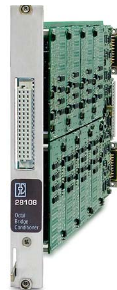
28108 Front Panel with Auxiliary Output Connector
