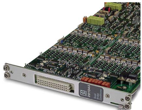
28104A Front Panel with Auxiliary Output Connector
