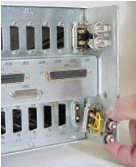
The 27000 chassis allows for a direct shielded coaxial connection to the 27304 input charge converter and the mating I/O cables to result in the lowest noise pickup. 27304 cards may be "hot swapped" from the front of the unit without disconnecting any rear panel cables.
